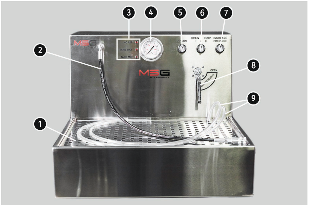
Figure 1. Main elements of the bench
