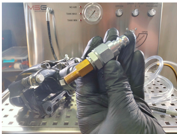
Figure 8. Connector and adapter matched to caliper threads
